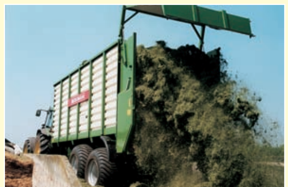
Scraper floor speed: 16.2 m/min at 1,000 rpm
